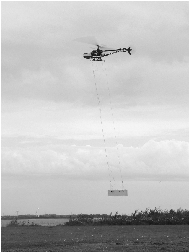
Fig. 17 Aalborg University Bergen Industrial Twin flying with dual-wire demonstration slung load.
